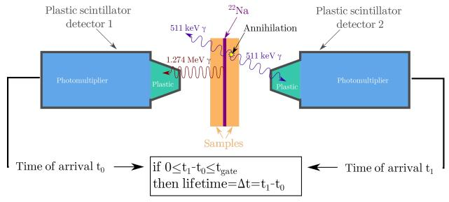
The positron is emitted first, nearly at the same time as the 1.274 keV photon which gives the start time (or  $t_0$ ). After some time, depending on the nature of the material and its defects, the positron will annihilate emitting two almost co-linear 511 keV photons. In case of standard double coincidence PALS measurements the detection of one of these
